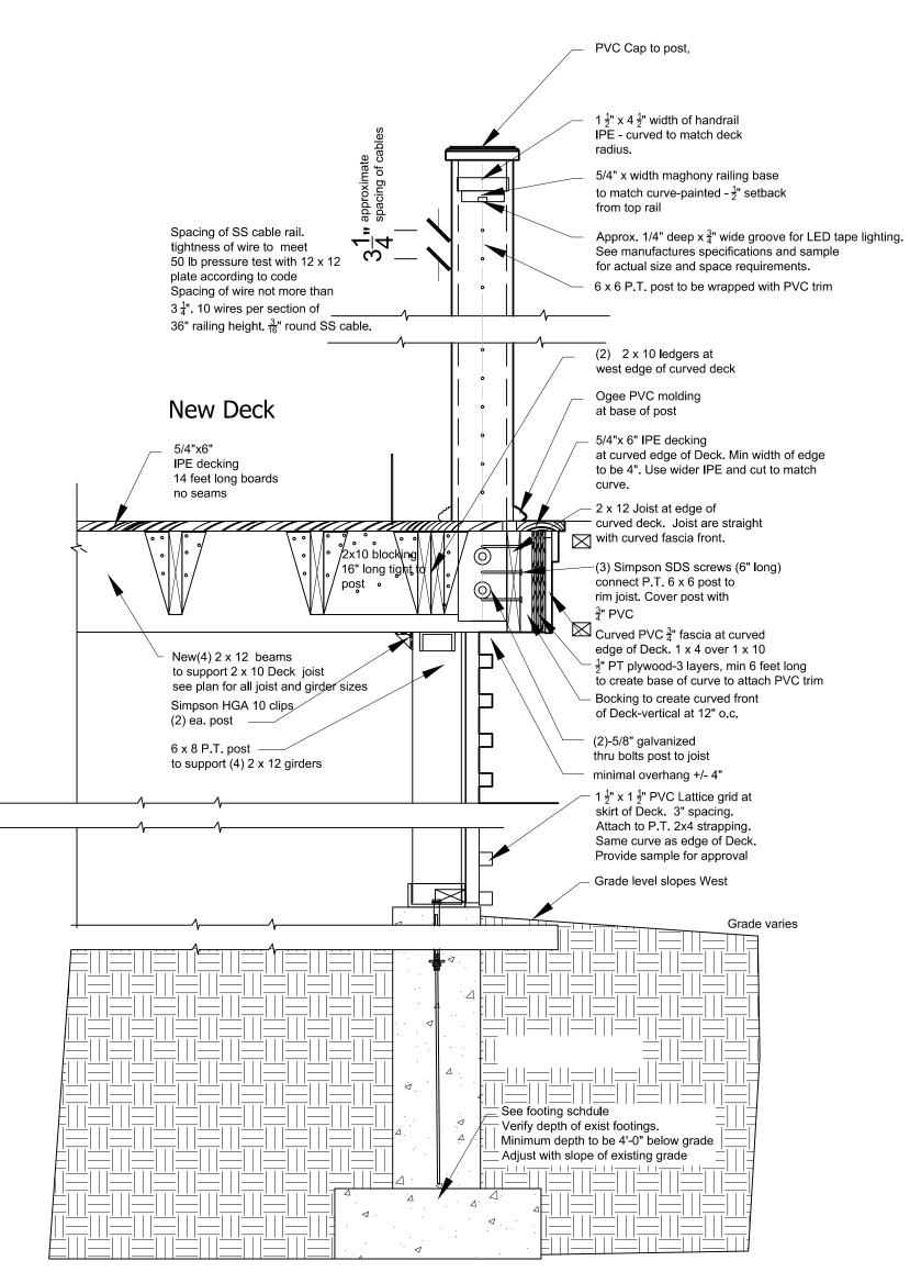
Section-B footings and Deck Railing
