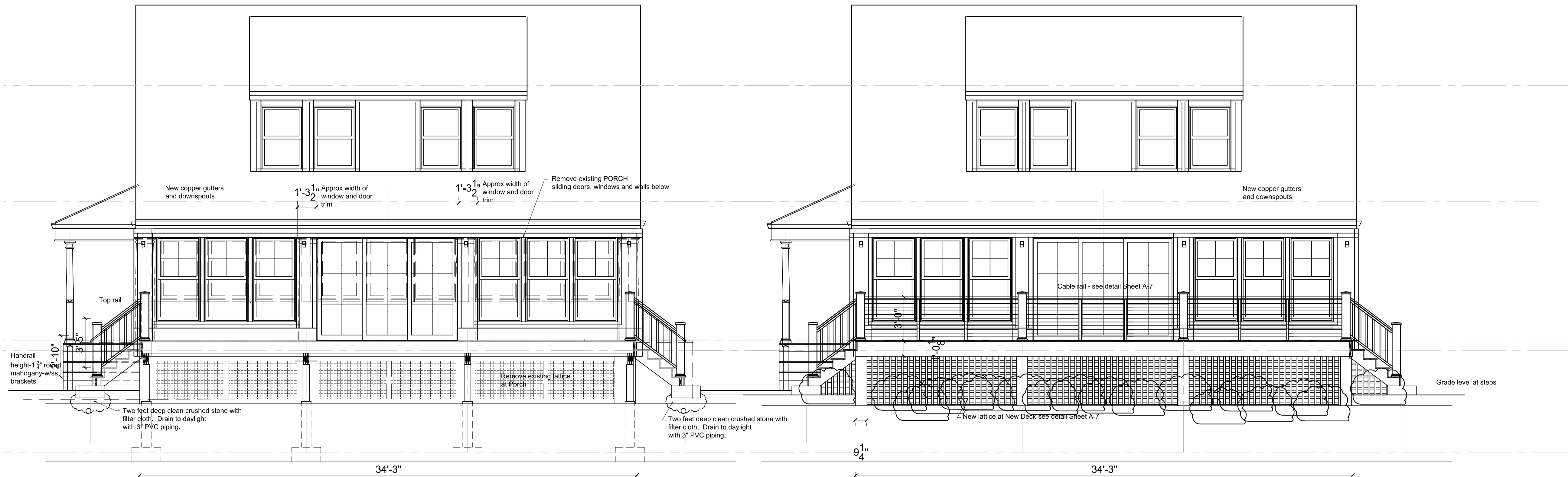
1 Elevation / Deck Section - West
