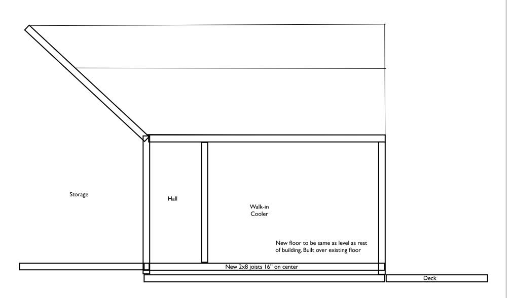
Revised pages 8 & 10 as per inspector review original 2x6 floor joists now 2x8 joists
