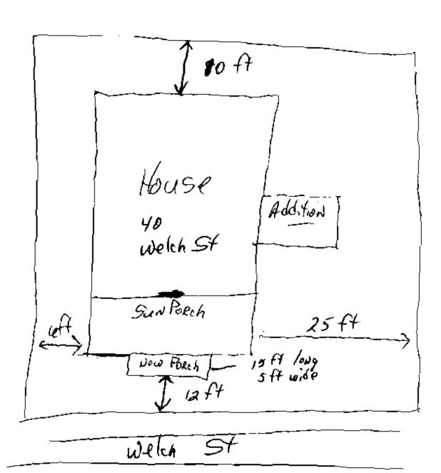
766-2421 Kockwell 40 Welch, St Veaks Island ME 2x 2 PT balusters 40° high - 484 PTV = 8" tabe 3-4 feet v AttAched to SUNROOM to preh Vastep steir Ty decking PT N7 /4 riser 110 1/2 treat composite Replacing existing deck New deck is shorter & farther from street
