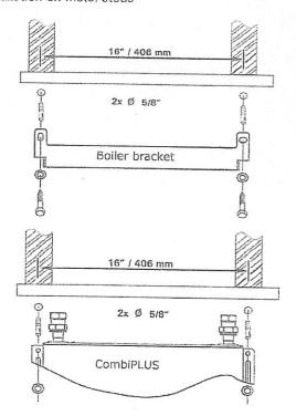
Install mounting bracket and CombiPLUS on wood studs as per illustration. Drill <sup>3</sup>/16" pilot holes to insert mounting bolts. Ensure that holes are located in the center of each wood stud. Secure with bolts to wooden studs as shown.
