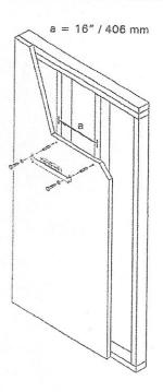
Install mounting bracket and CombiPLUS on metal studs as per illustration. Drill %" pilot holes to insert anchors. Ensure that holes are located in the center of each metal stud. Use appropriate fasteners to mount CombiPLUS to metal studs (not supplied). Secure with bolts to metal studs as shown.
