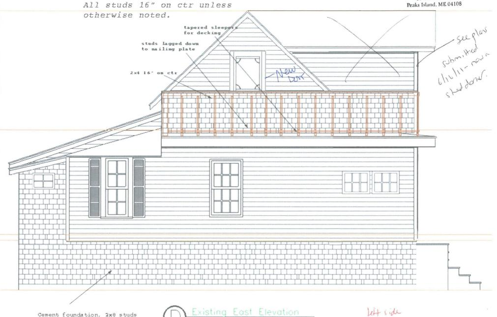
Cement foundation, 2x8 studs on an 0x0 house sill plate.
