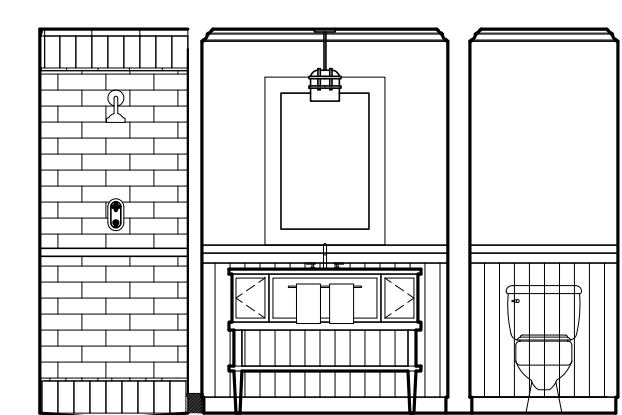
12 INTERIOR ELEVATION UNIT 213 1/4"=1'-0"
