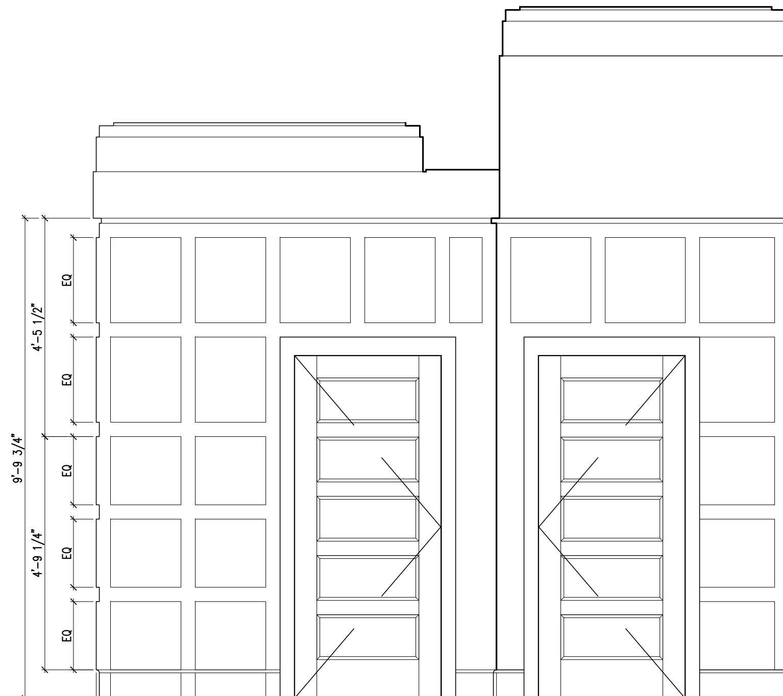
12 INTERIOR ELEVATION AT ELEVATOR LOBBY 1/2"=1'-0"
