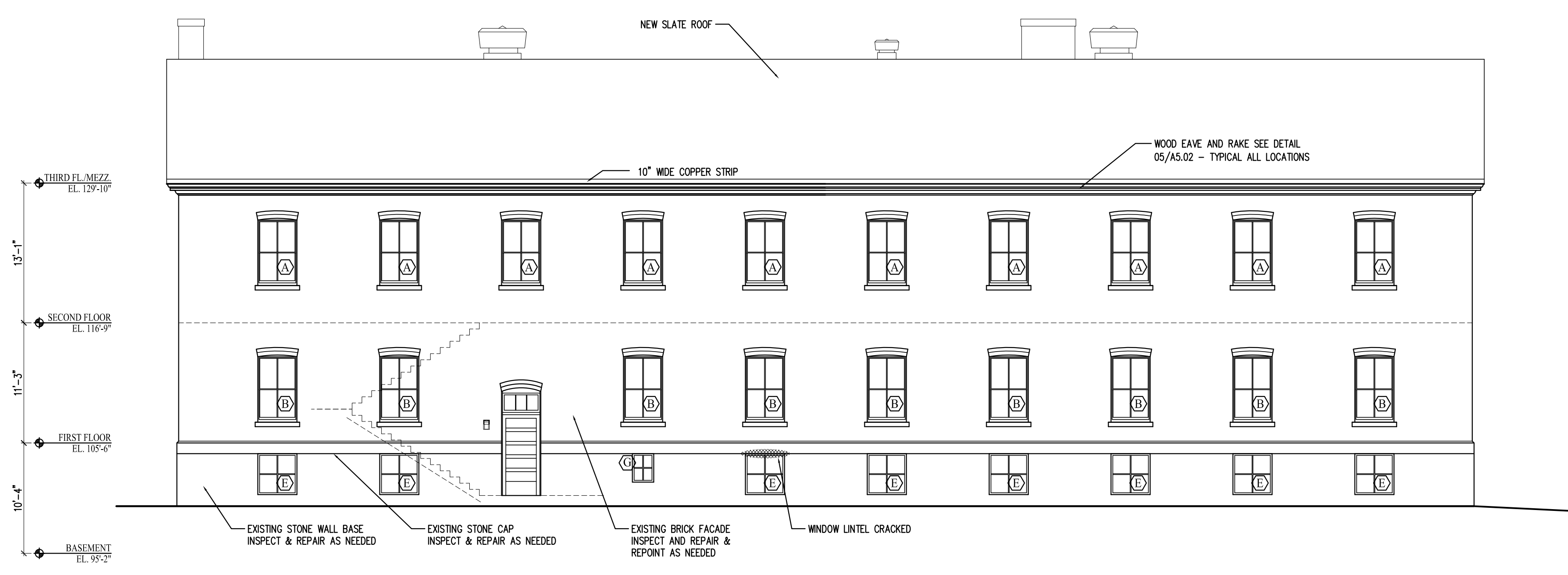
4 | WEST ELEVATION - ADDITION SCALE: 1/8"=1'-0"
