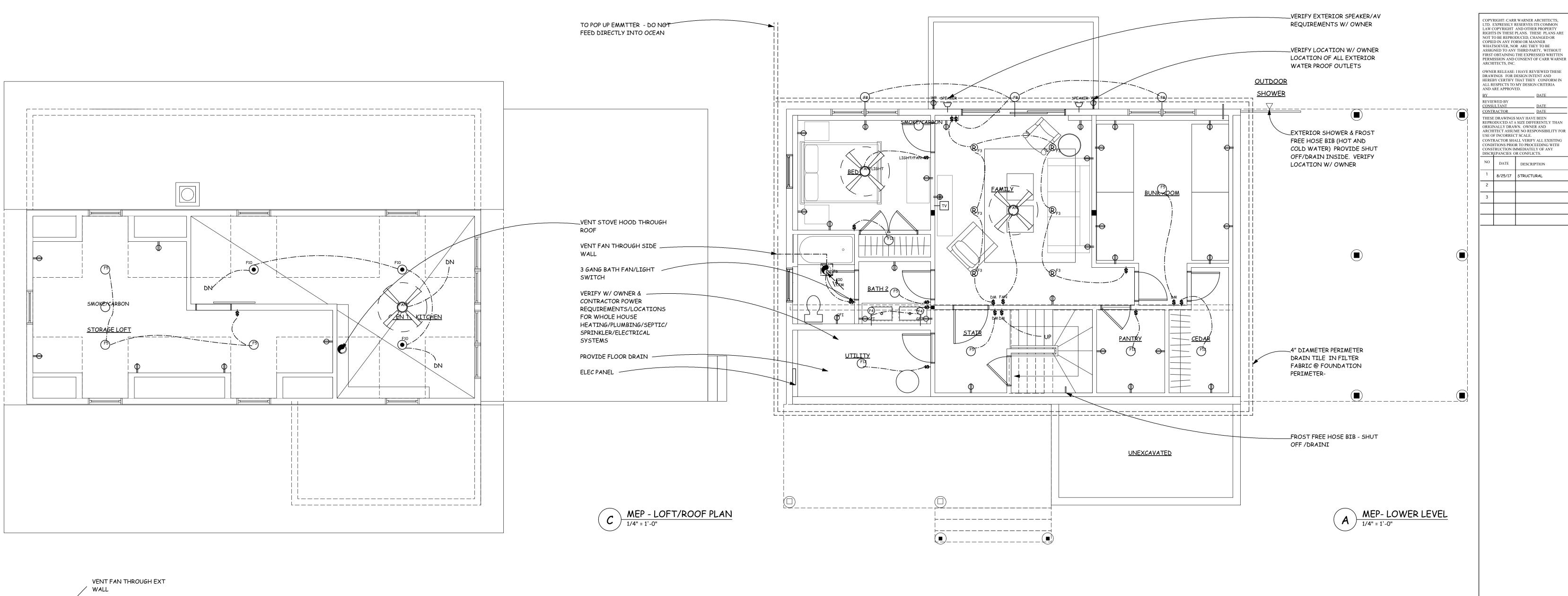
1. AFCI PROTECT LIGHTS AND OUTLETS PER NEC 210.12(B)
