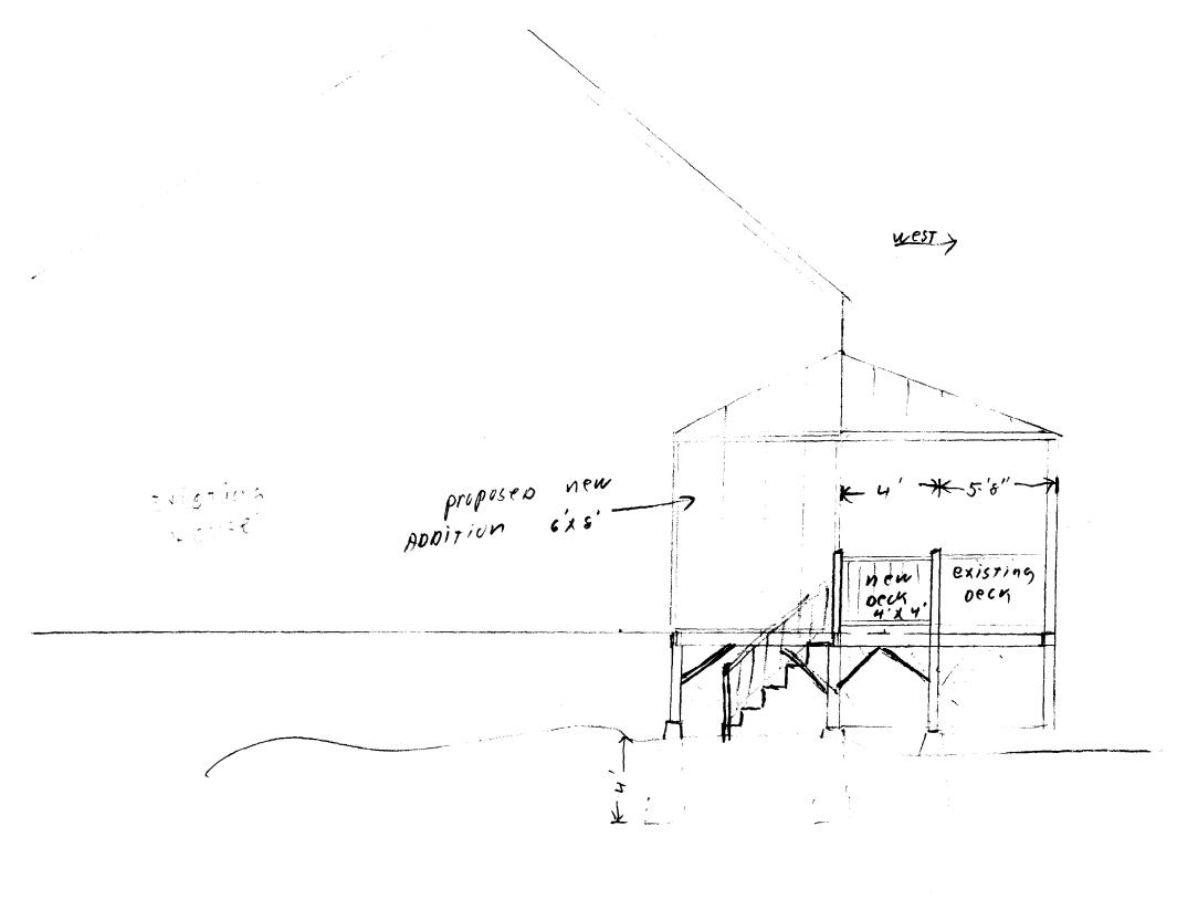
, o Base r perimeter iexisting 216. goist 2+89<sup>7</sup>8". Tape, id Je (Vire) peck y`x4' pathroom existing buth addition 6'x8' door, uxs" header 1 4'X8' 2xx joist 16" oc doubled at 6×6 posts p.T. perimeter Tapered concrete columns @ 10" base 2×8 Wender to new! 4' deep anchers, 5/4 subfluer w 1/2" under lang ment Hip roof @ 2x8 hip rafter and 2x6 raflers 16" oc 34's heathing. 224 mall construction 16" O.C. HOUSE 31' X 35' double top plate, 3/4"sheathing
