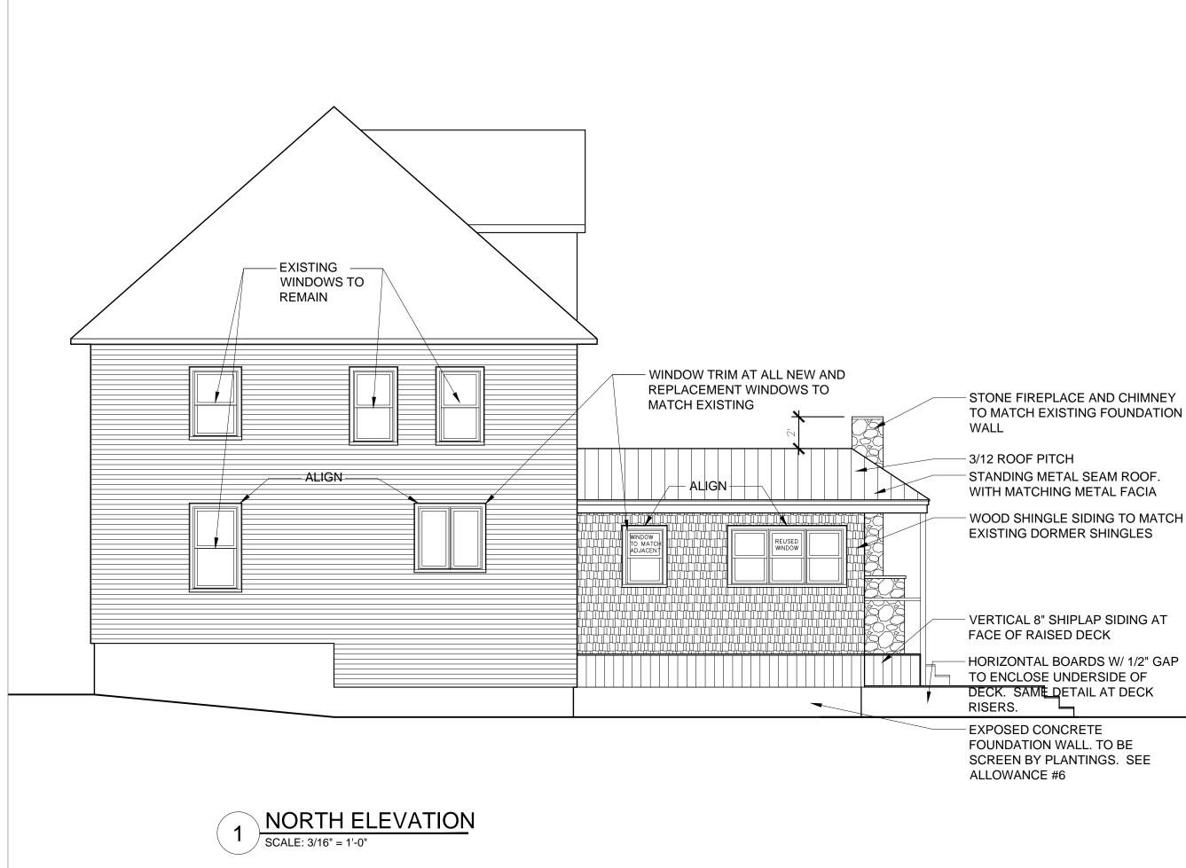
EXPOSED CONCRETE FOUNDATION WALL. TO BE SCREEN BY PLANTINGS. SEE
