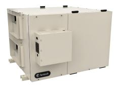
The SHR 6904 Commercial Heat Recovery Ventilation system (HRV) complements today's tight buildings. Fantech Heat Recovery Ventilators (HRV) are designed to supply air into a building while exhausting an equal amount of contaminated air to the outside. The aluminum heat exchanger core transfers sensible energy between air streams resulting in tempering of the supply air and reduced loads on the HVAC system.
