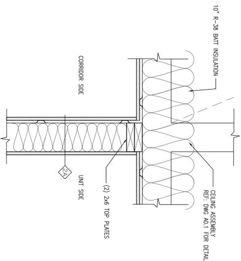
A7.1 INTERIOR BEARING WALL DETAIL
