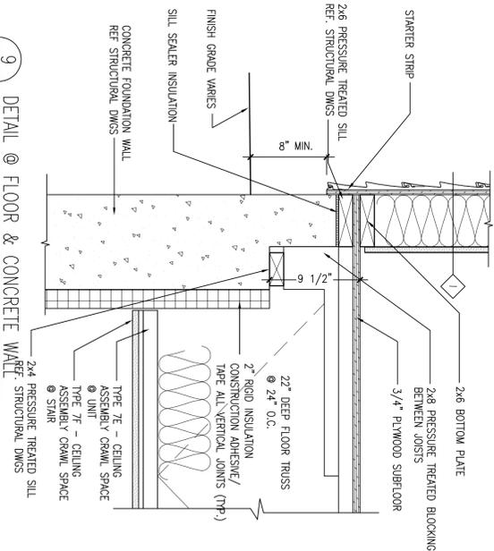
A7.1 DETAIL @ FLOOR & CONCRETE WALL
