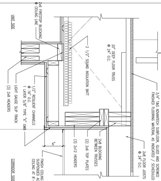
A7.1 DETAIL @ FLOOR & EXTERIOR WALL
