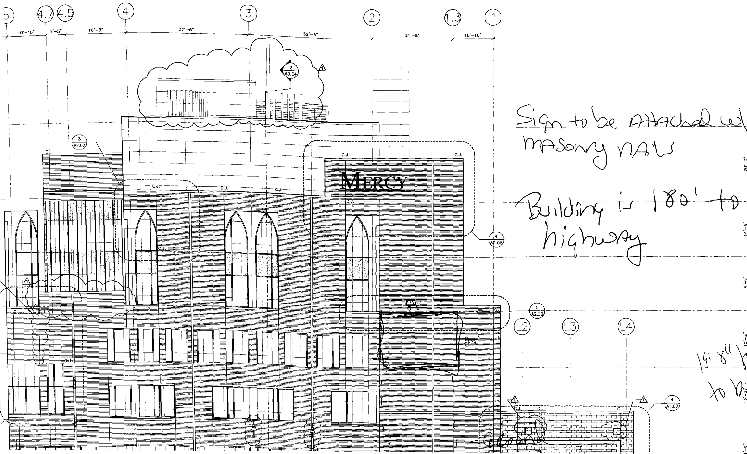
COURSING DETAIL - PARTIAL SOUTH ELEVATION SCALE: 1/8"=1'-0"
