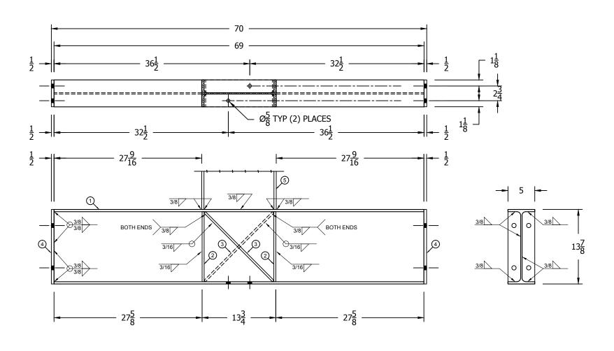
W14 X 26# X 70" DOUBLE SIDED CANTILEVER BASE STANDARD TOLERANCES
