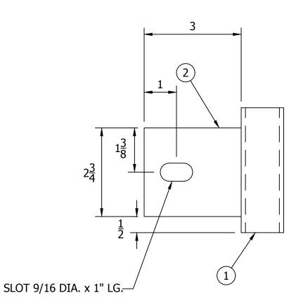
POLE SOCKET FOR 4" & 5" ARM HALF FILE NAME: X-S-PIPE SOCKET FOR 4-5 INCH ARM.dwg
