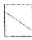
Type 4 Diagonal fracture with no cracking through caps; top with horizontal displacement from Type 1.
