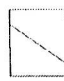
Type 4 Diagonal fracture with no cracking through caps, top with hammer to distinguish from Type 1
