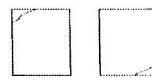
Type 5 Chips fractured at top or bottom faces or externally with substantial chips
