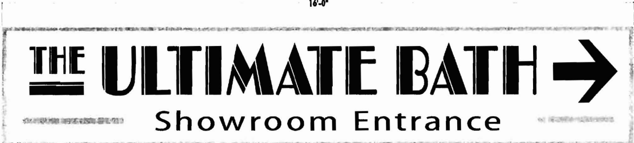
C ( ONE ) 3' x 16' S.F. NON-ILLUMINATED SIGN BAKED ENAMEL ALUMINUM FACES W/ 1" FRAME AND 1-1/2" ALUMINUM MOLDING
