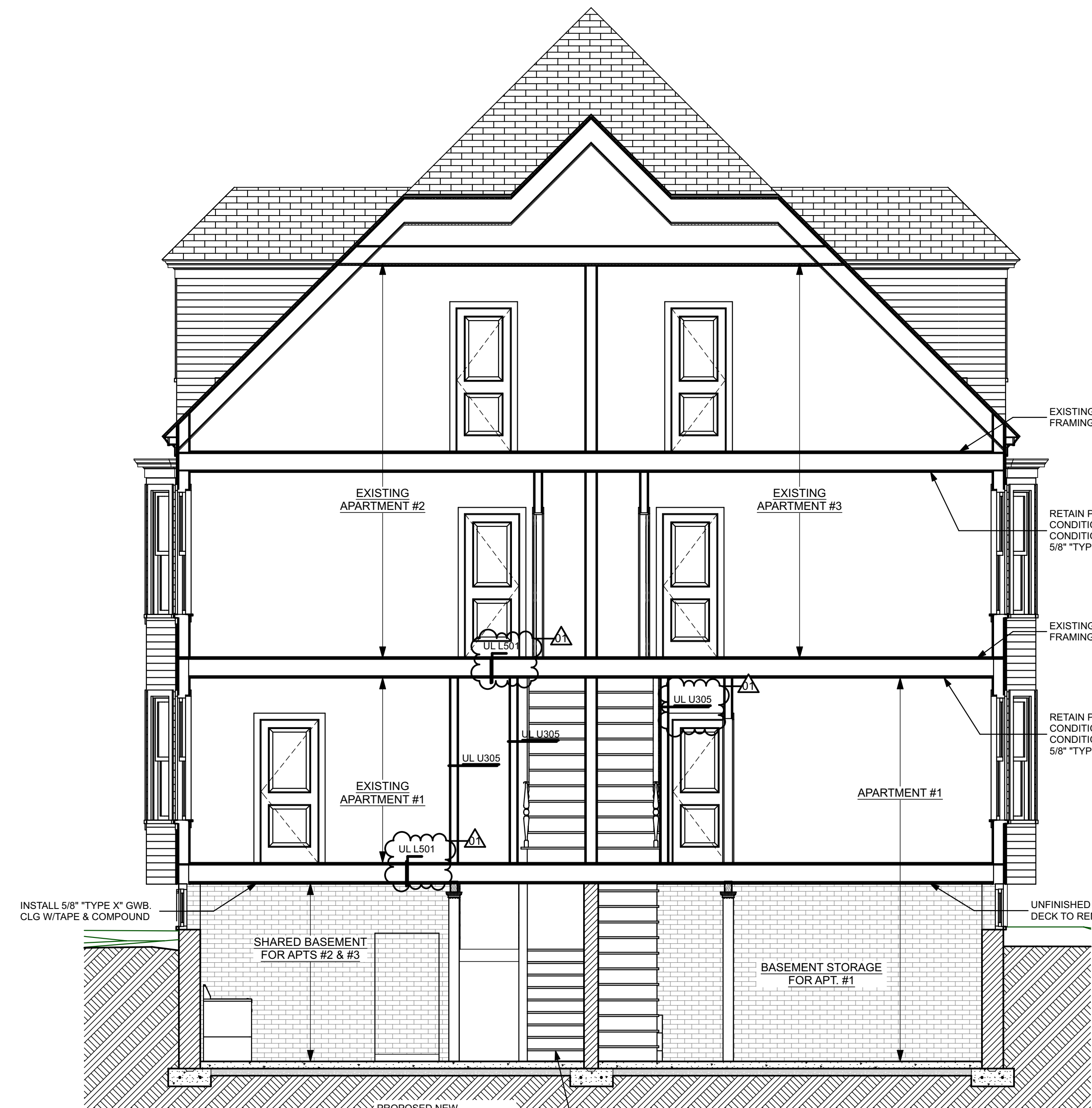
1 BUILDING SECTION A3.1 SCALE: 1/4" = 1'-0"
