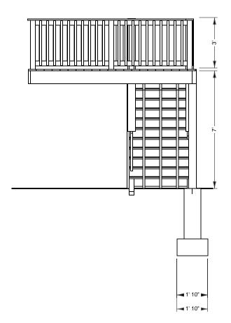
2x10 Ledger Board to be flashed and bolted (2) 1/2" bolts with washers or equivalent every 16" on center. (See ledger detail deck construction guide)
