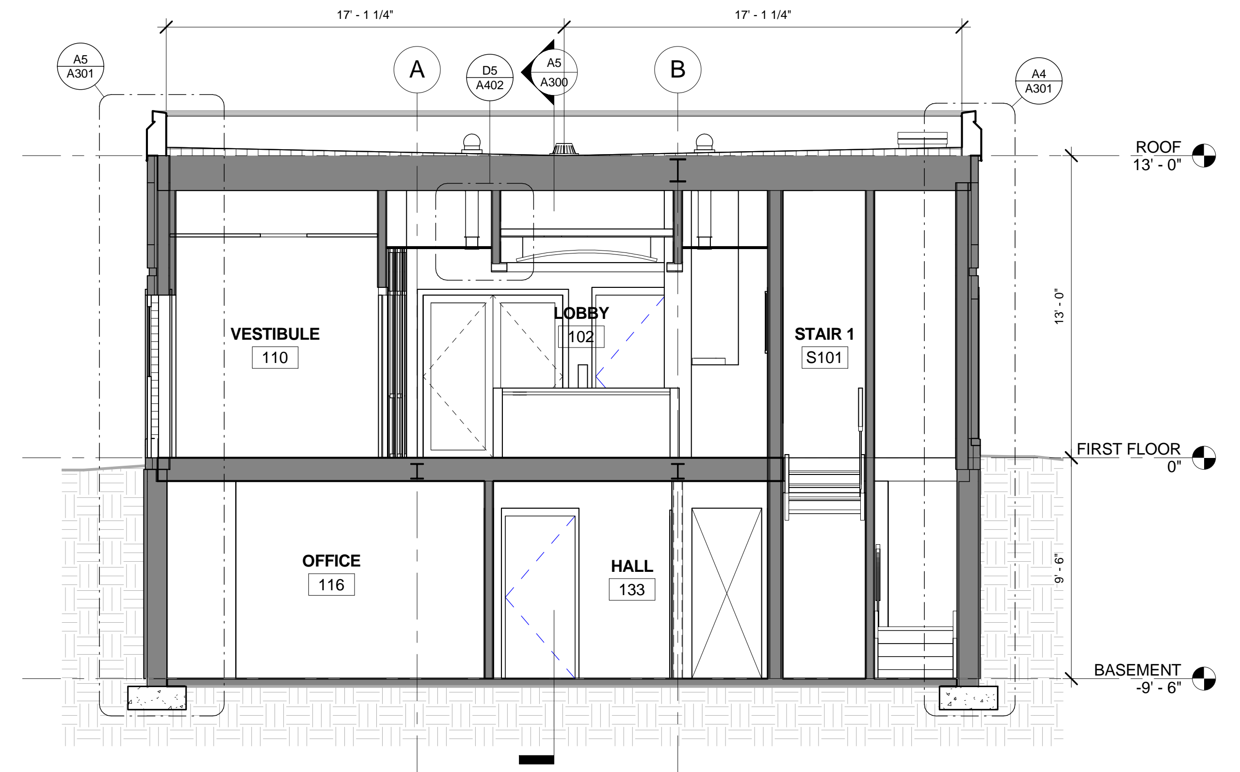
C3 EAST/WEST BUILDING SECTION 1/4" = 1'-0"
