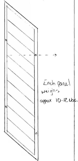
Note: Thunder boths are expanding Lags which do not require a lead shield ... The Yu" Lags would be screwed into a lead Lag shield inserted into sione race of building.
