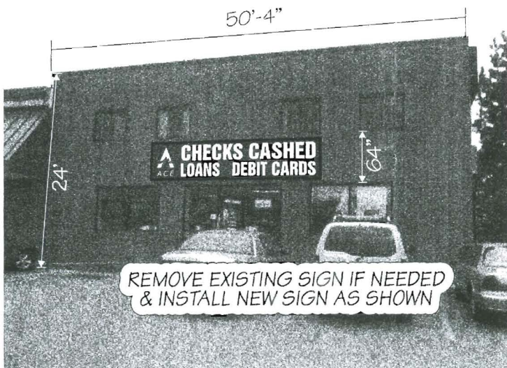
FRONT ELEVATION (AFTER)
