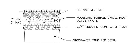
1. SUBBASE GRAVEL LAYER VARIES WITH FINISHED GRADE
