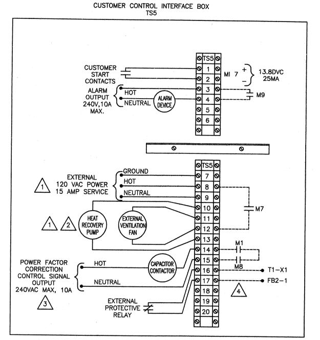
THE TECOGEN CAN START/STOP BOTH THE HEAT RECOVERY PUMP AND AN EXTERNAL VENTILATION FAN. POWER FROM AN OUTSIDE SOURCE MUST BE BROUGHT IN. IF POWER FOR BOTH DEVICES DOES NOT EXCEED 120 VAC, 15 AMPS, THEN THESE DEVICES CAN BE POWERED DIRECTLY FROM THE MODULE OUTPUTS. OTHERWISE THE OUTPUT TO ENERGIZE THE MOTOR STARTERS.
