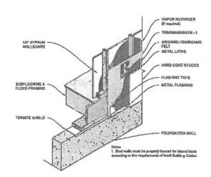
Re-Siding Construction - Thermasheath-3 may be used in retrofit construction provided the existing siding is sound and solidly attached. It is secured with galvanized nails of sufficient length to penetrate the old sidings, sheathings below and at least one inch into the existing wall studs. Then, cover the Thermasheath-3 with a suitable new siding of aluminum, vinyl, fiber cement, wood or wood fiber based products.
