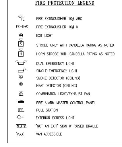
1. ALL EMERGENCY LIGHTS MUST BE POWERED BY BATTERY BACK-UP <u>OR</u> GENERATOR PER NFPA 101. 2. HVAC PER NFPA 90A 3. EMERGENCY LIGHTS TO AVERAGE 1 FOOTCANDLE AND .1 FOOTCANDLE MINIMUM.
