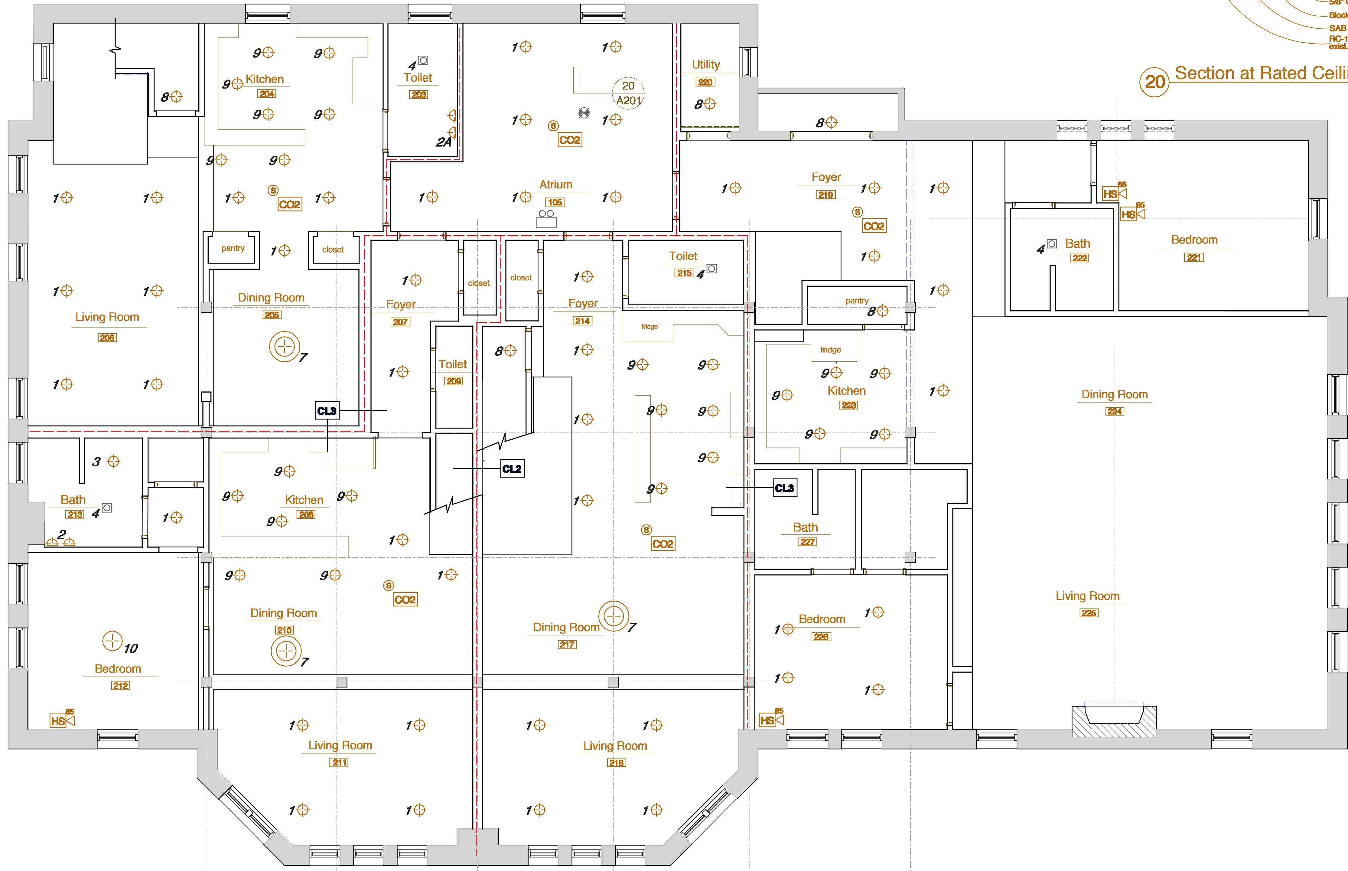
10 Second Floor Reflected Ceiling Plan
