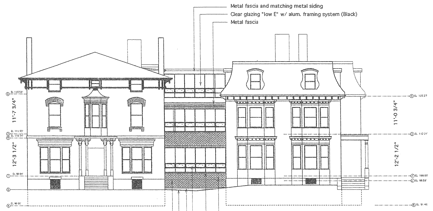
North Elevation Study SPRING STREET 6/3/99
