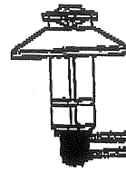
SAP1 ARM MOUNT FOR SP1 Designed to slip over a 4"/100mm diameter pole.
