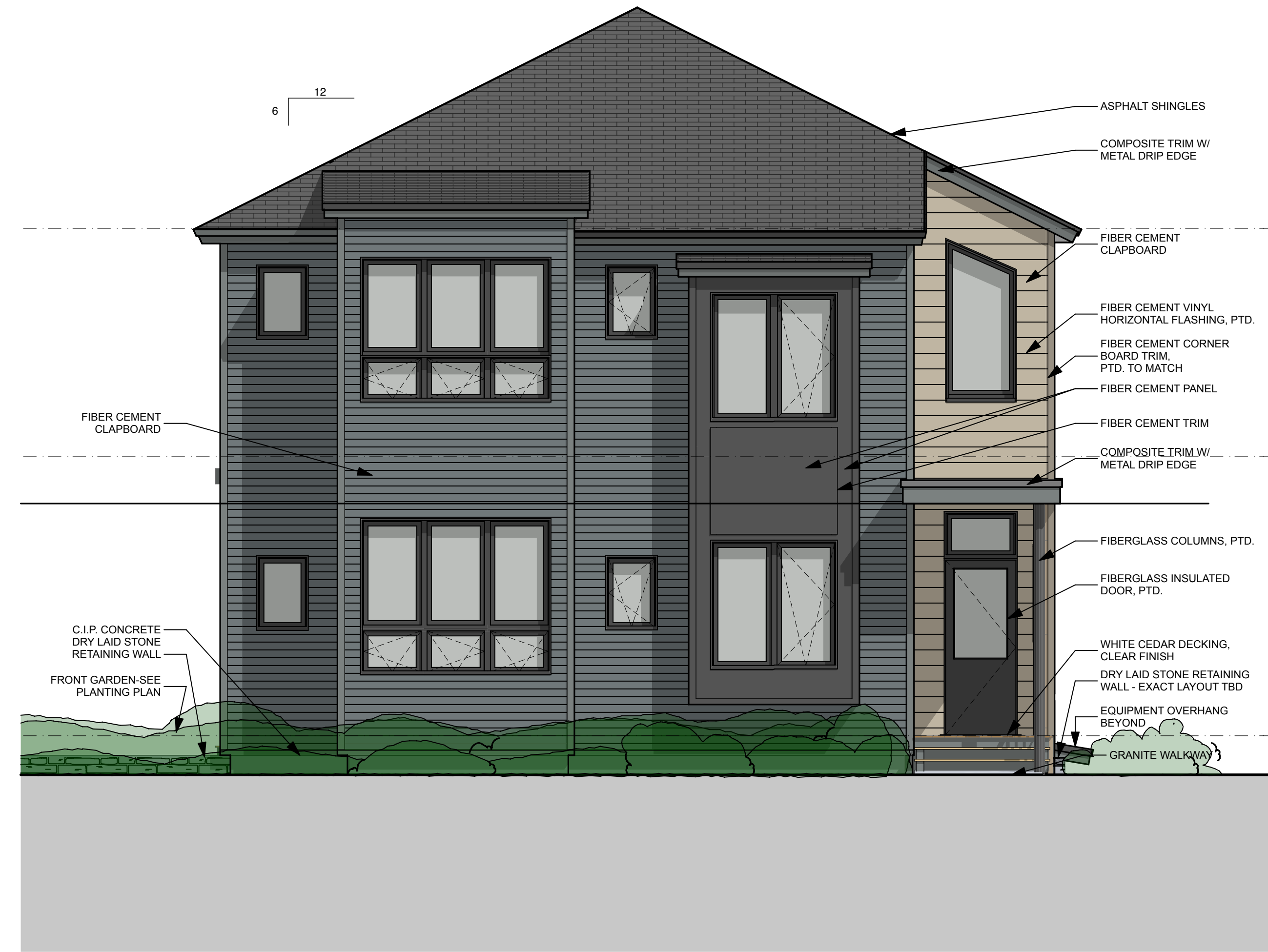
1 NORTH ELEVATION: DANFORTH ST. SCALE: 1/4" = 1'-0"
