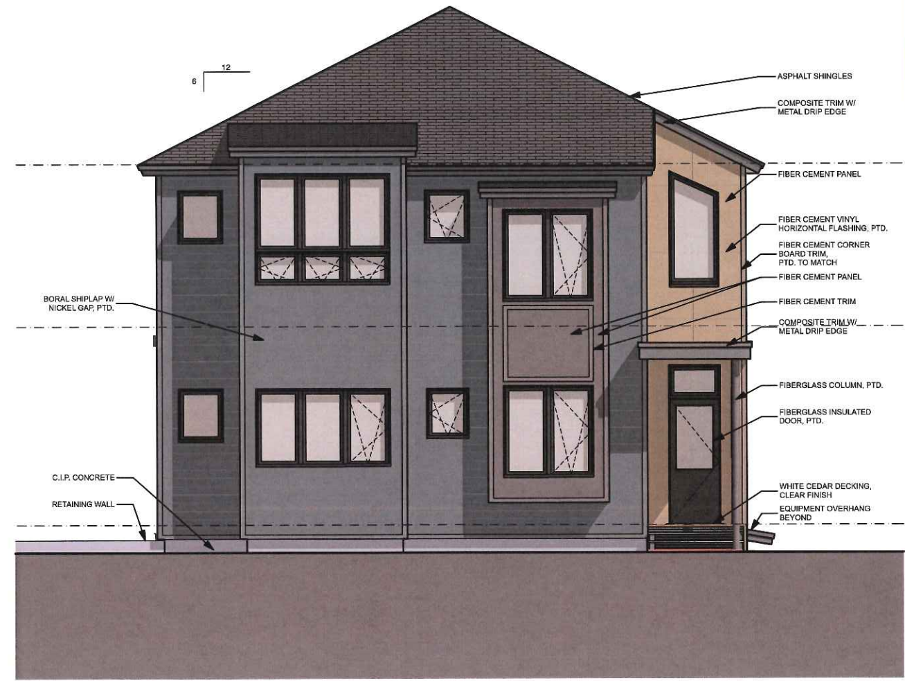
1 NORTH ELEVATION: DANFORTH ST. SCALE: 1/4" = 1'-0"
