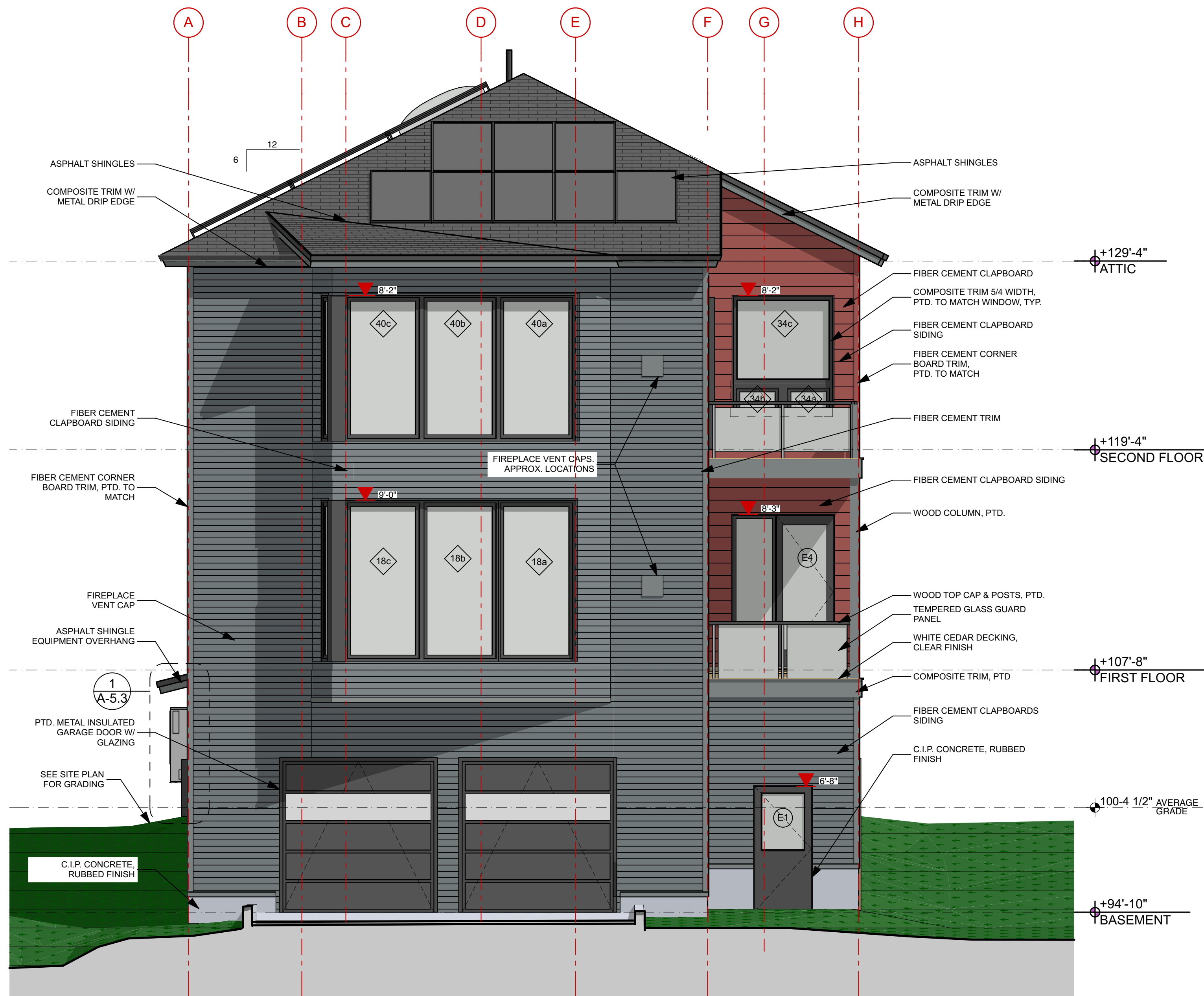
2 SOUTH ELEVATION SCALE: 1/4" = 1'-0"
