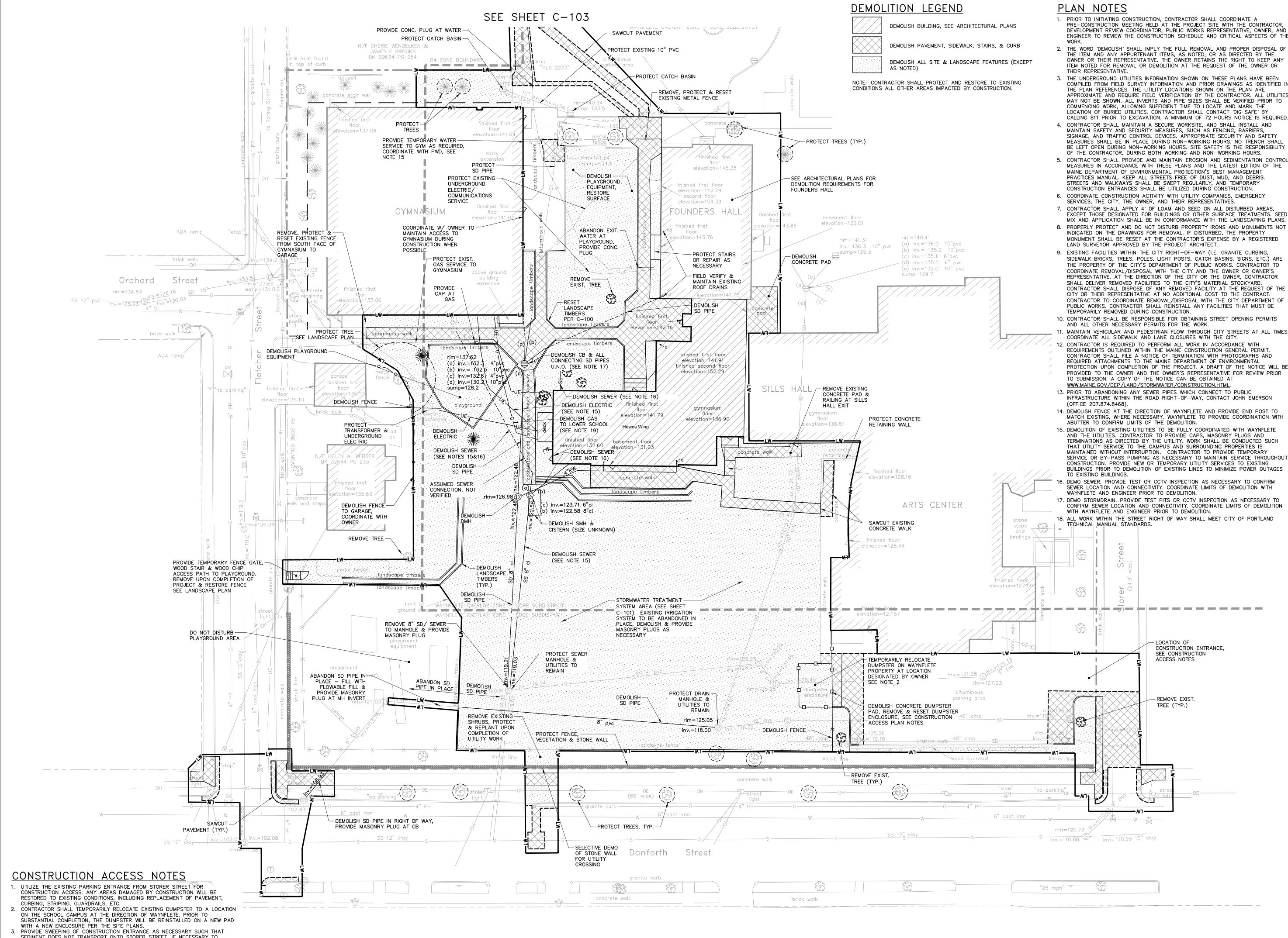
SEDIMENT DOES NOT TRANSPORT ONTO STORER STREET. IF NECESSARY TO CONTROL SEDIMENT, CONTRACTOR TO PROVIDE TEMPORARY CONSTRUCTION ENTRANCE PER DETAILS ON SHEET D-203.
