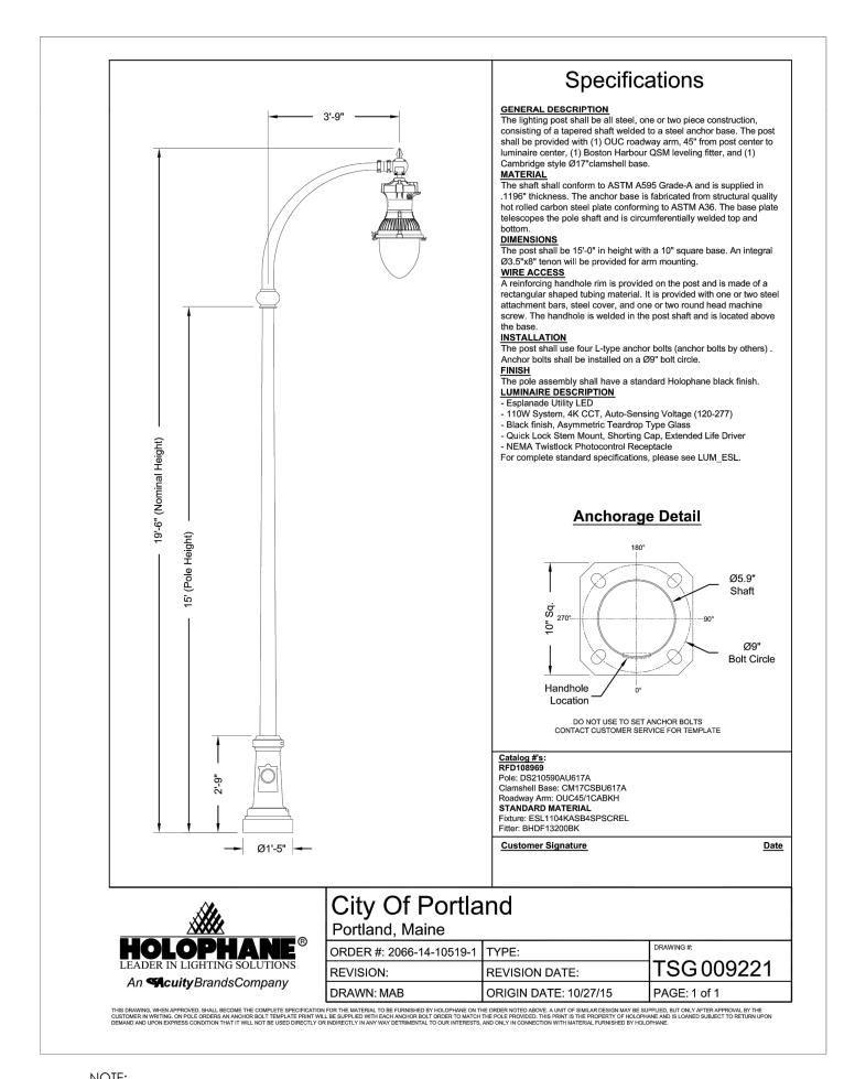
1. LED FIXTURES, 3000k, BLACK IN COLOR (BASE, POLE LIGHT FIXTURE), CONCRETE BASE SET 2" TO 4" ABOVE FINISH GRADE.
