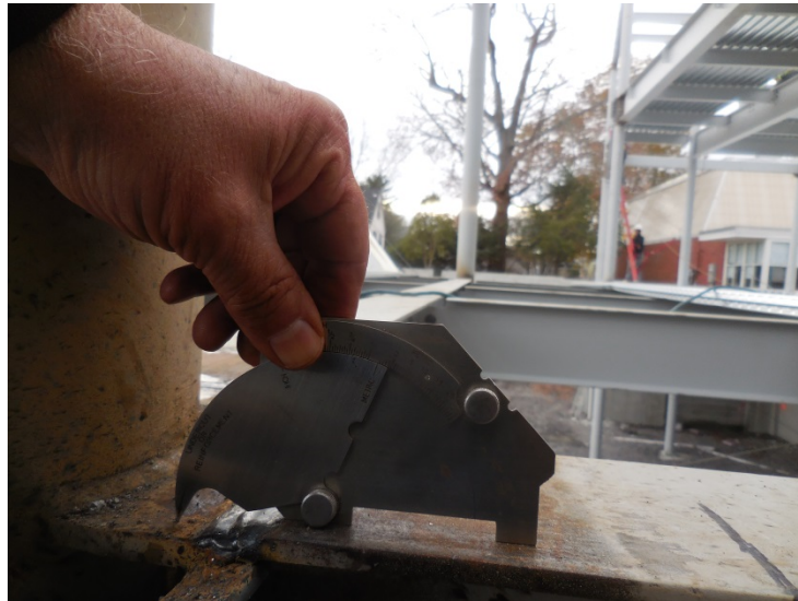
Cam gage used to measure misalignment
