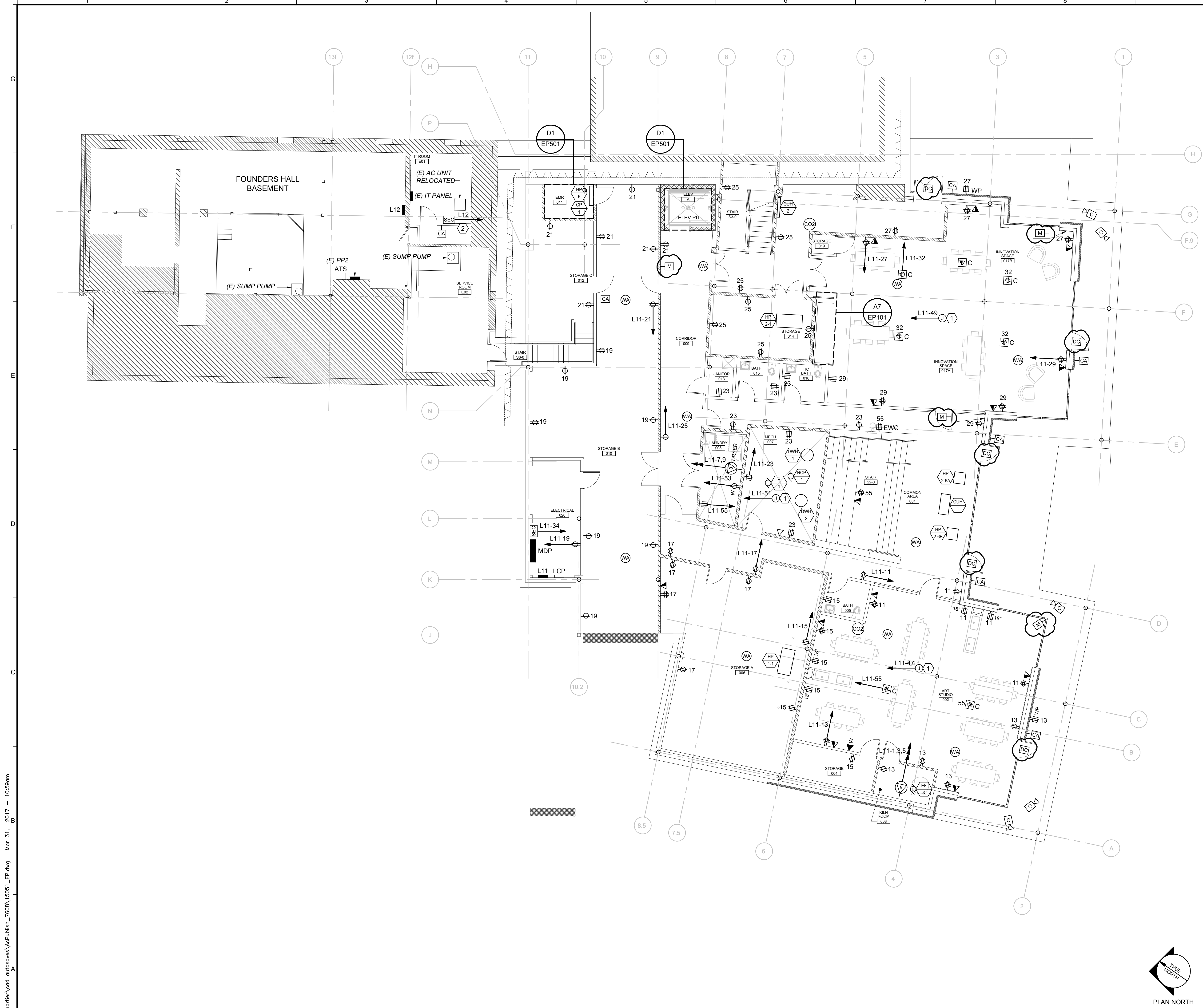
A1 POWER AND SYSTEMS PLAN ~ LOWER LEVEL 1/8" = 1'-0"
