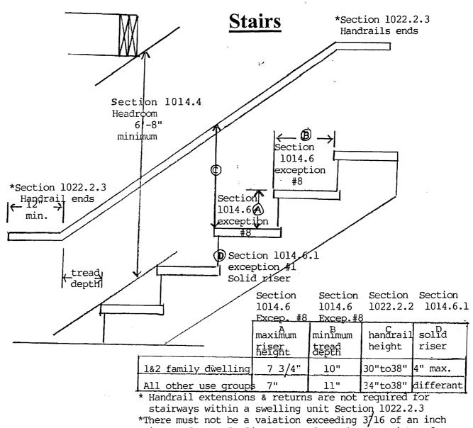
in the depth of adjacent treads or in the height of adjacent risers. Section 1014.6.2
