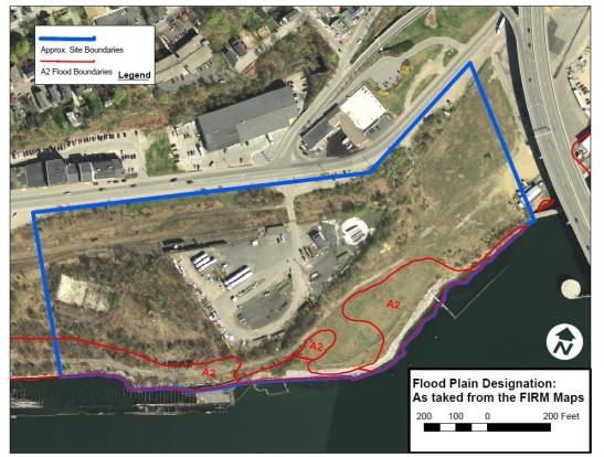
Portland's Flood Plain Management ordinance requires buildings within "A" flood zones have finished floors more than 2 feet above the base flood elevations. The proposed development is showing a minimum of elevation 13 for finished floors and is compliance with this provision
