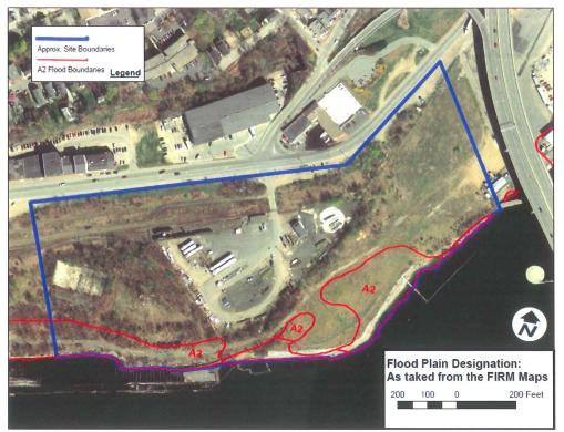
Portland's Flood Plain Management ordinance requires buildings within "A" flood zones have finished floors more than 2 feet above the base flood elevations. The proposed development is showing a minimum of elevation 13 for finished floors and is compliance with this provision
