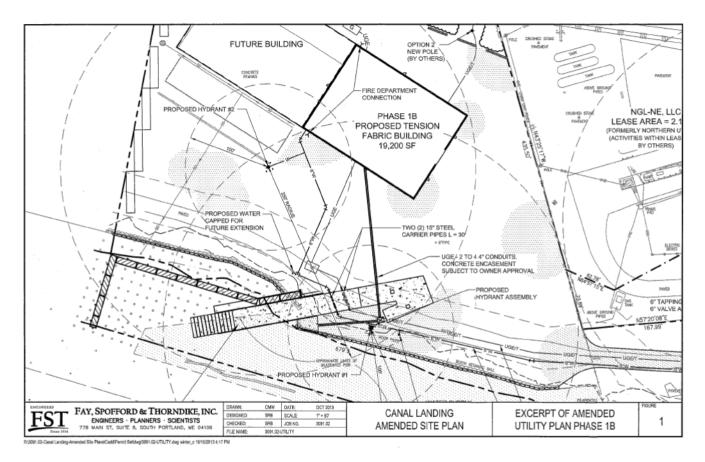
The site is currently served by two fire hydrants on West Commercial Street and an additional hydrant in the interior of the site. The proposed utility plan, Attachment P10, (excerpted above) shows additional hydrant locations within blue buffer circles.
