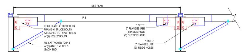
TYPICAL P-3 BRACE DETAIL SCALE: 3/4" = 1'-0"
