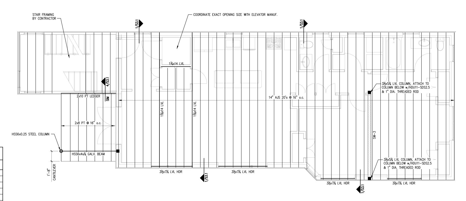
SHEAR WALL SCHEDULE BETWEEN FLOOR DIAPHRAGMS SHEATHING NAILING AT GRID REQUIREMENTS PANEL EDGES REMARKS SW-3 ONE SIDE 3" o.c. SW-3B BOTH SIDES 3" o.c. SW-4 ONE SIDE 4" o.c. SW-4B BOTH SIDES 4" o.c. SW-6 ONE SIDE 6" o.c. SW-6B BOTH SIDES 6" o.c.
