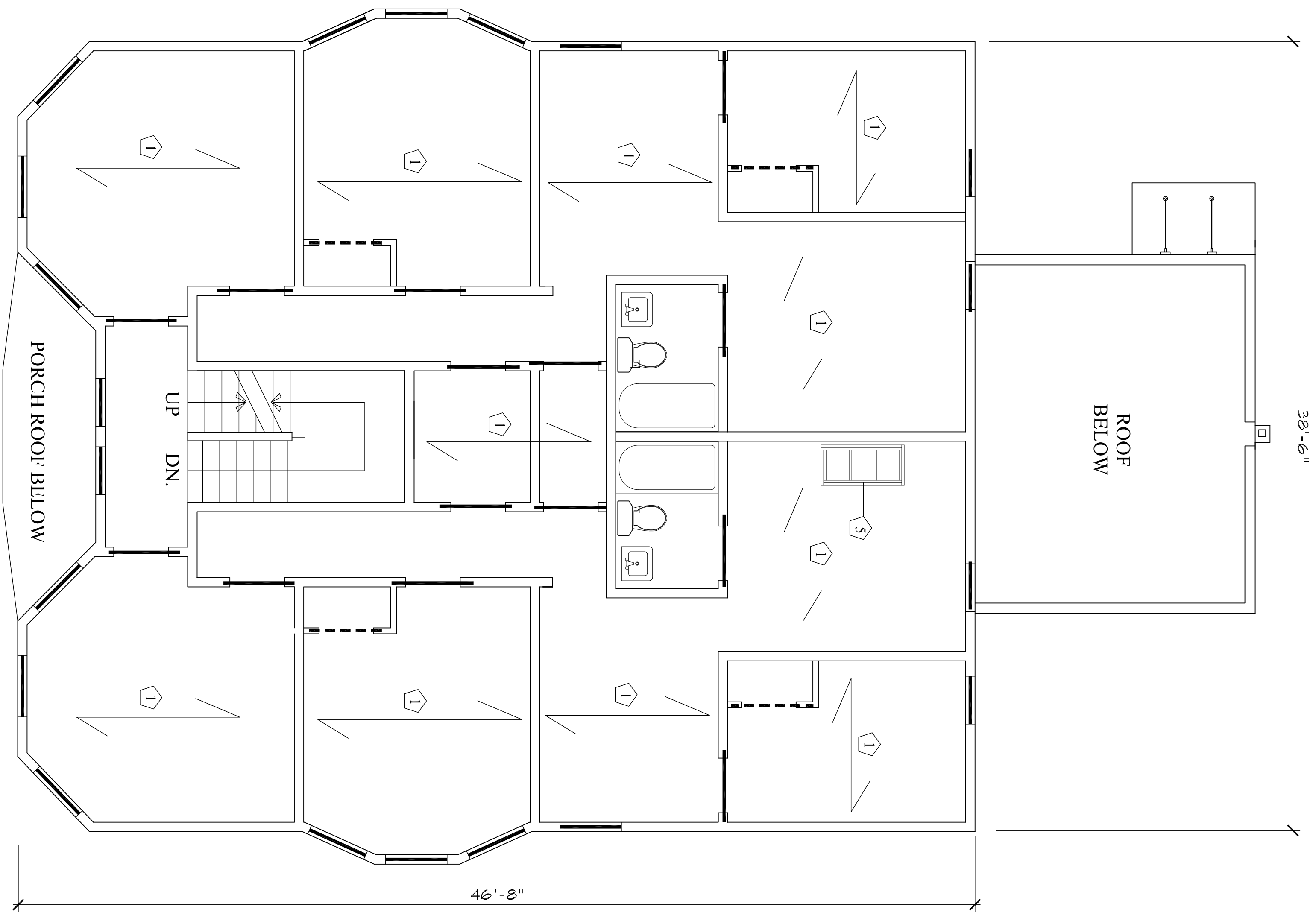
2 THIRD FLOOR FRAMING PLAN 1/4" = 1'-0"
