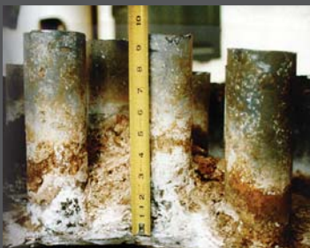
Traditional tank-type water heater flue tubes with nearly 6" of lime scale buildup
