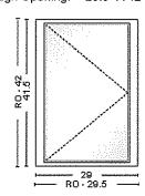
0171-New Construction Right 29 x 41.5 Operation / Venting = Right New Construction With J-Channel Frame Color = White CLIMATECH, No Upgrade Egress Hardware U-Factor = 0.28, CR = 59, SHGC = 0.28, VT = 0.5, CPD = ASO-A-31-04063-00001 No Jamb Extension, NC Wrapping, Rough Opening Line Item Notes:
