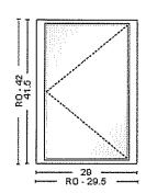
0171-New Construction Left 29 x 41.5 Operation / Venting = Left New Construction With J-Channel Frame Color = White CLIMATECH, No Upgrade Egress Hardware U-Factor = 0.28, CR = 59, SHGC = 0.28, VT = 0.5, CPD = ASO-A-31-04063-00001 No Jamb Extension, NC Wrapping, Frame Size Line Item Notes:
