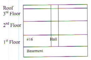
The wall to be removed is a bearing wall, taking roof, third floor and second floor loads from the hall and the room. The hall is assumed to be present with bearing walls on either side on all the floors, and the roof is assumed to also be supported at this wall.
