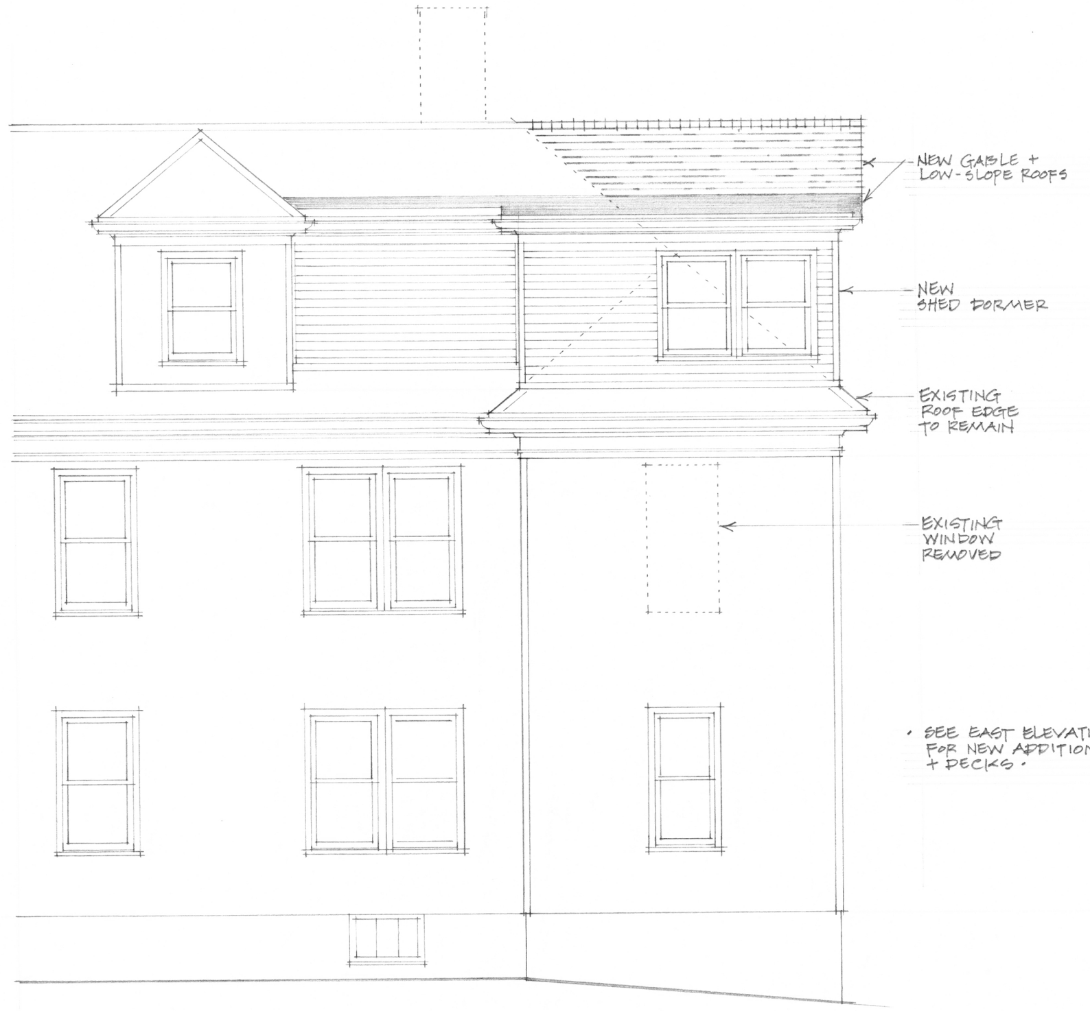
WEST ELEVATION - (PARTIAL)
