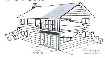
This table provides CP-LAM header sizes for the support of one level of floor framing, an exterior wall and roof trusses over various rough openings. A 2 foot maximum roof overhang and center support for the floor framing are assumed.
