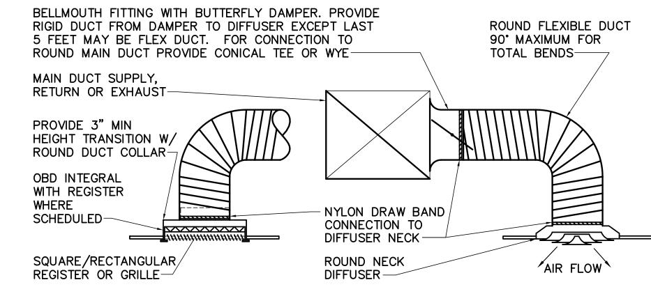
4 DIFFUSER AND REGISTER RUNOUT DETAIL M-001 NOT TO SCALE
